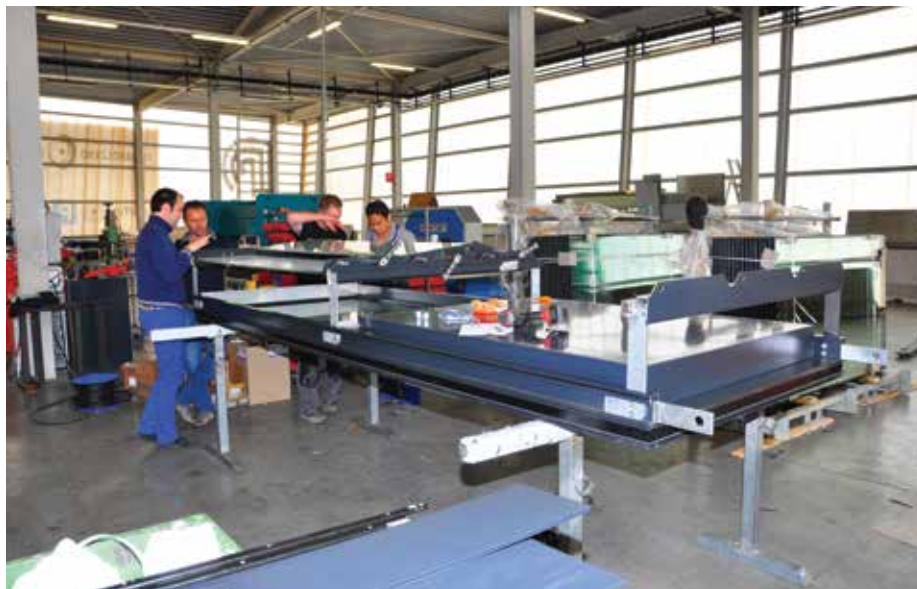
Figure 6. Modular façade with optimized interfaces and standardized functional principles (Media Banca, Milan, Italy). (Source: Schueco International KG)
