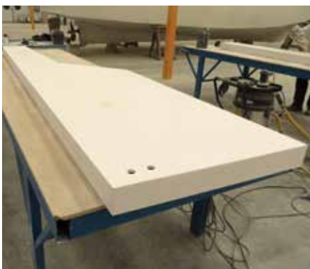
Figure 12. A fin with the two half-shells joined (Source: ENvolventes ARquitectonicas - ENAR)
