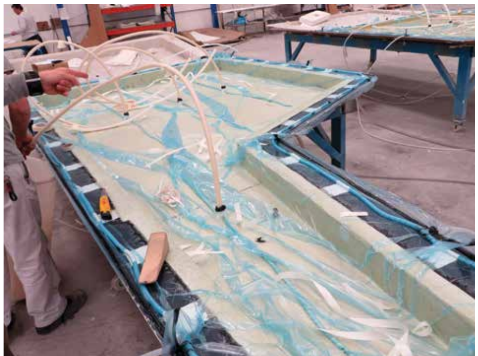
Figure 10. Infusion process (Source: ENvolventes ARquitectonicas - ENAR)
