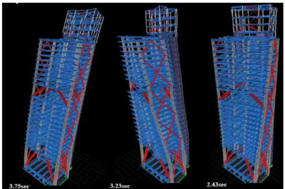
Figure 9. Fundamental dynamic mode shapes (Source: Arup)
