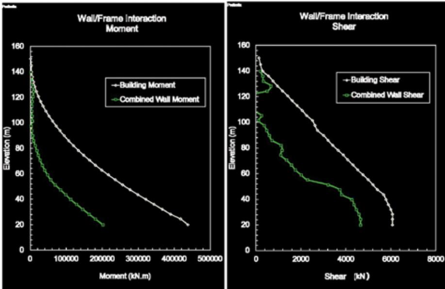
Figure 4. Distribution of moment and shear between the cores and braced frames under wind loading in the north-south direction (Source: Arup)
