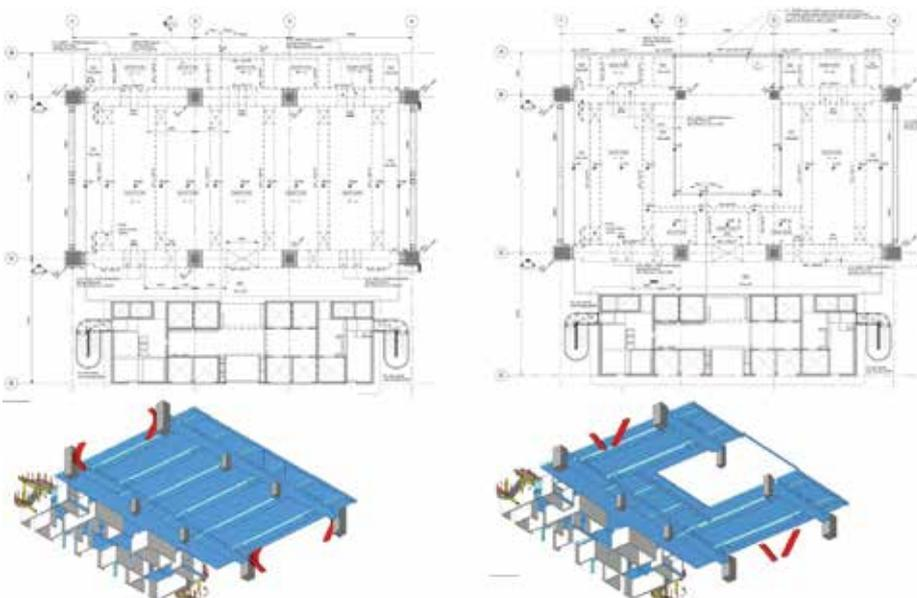
Figure 3. Typical floor structure. Full floor (left) and village floor (right). 3D views from below under (Source: Arup)
