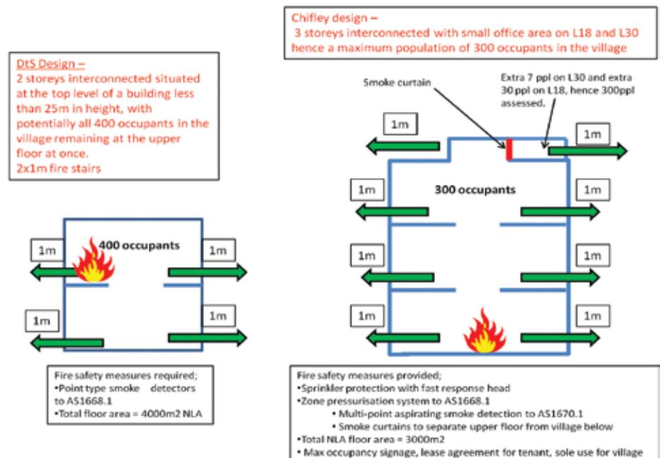
Figure 13. Comparison of 8 Chifley to DTS interconnection criteria (Source: Arup)
