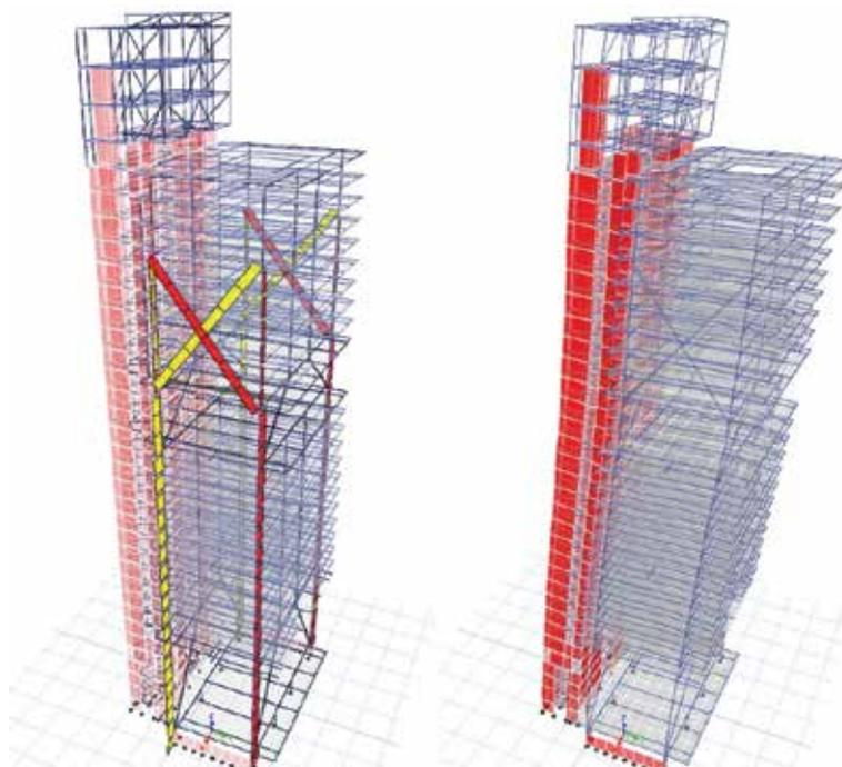
Figure 6. Structural analysis under fire load case with Zone 2 fire condition (Source: Arup)
