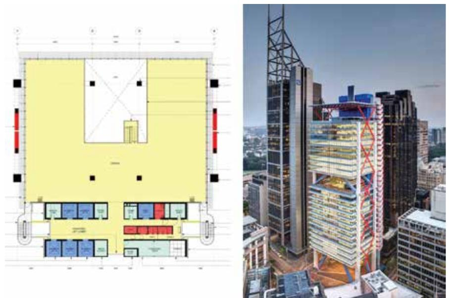
Figure 1. Typical village floor plan at architectural concept, and completed building. Only two columns are located within the floorplate on the village floors (Source: RSHP & Brett Boardman)
