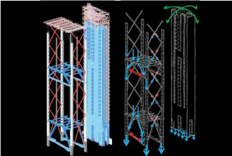
Figure 2. Stability and Gravity System (Source: Arup)
