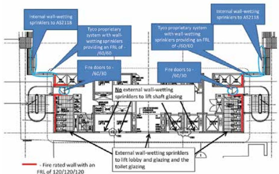
Figure 12. Fire separation to external stairs (Arup)
