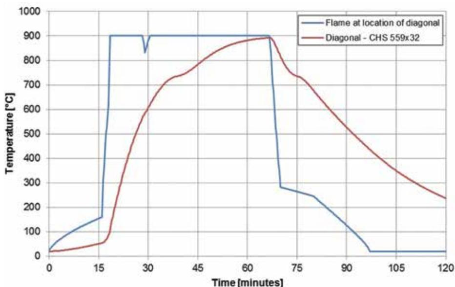
Figure 7. Flame and diagonal temperature 1m above the roof of the vehicle (Source: BuroHappold Engineering)
