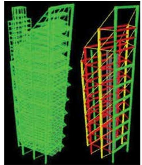
Figure 8. ETABS Structural FE model and stability members only model (Source: BuroHappold Engineering)
