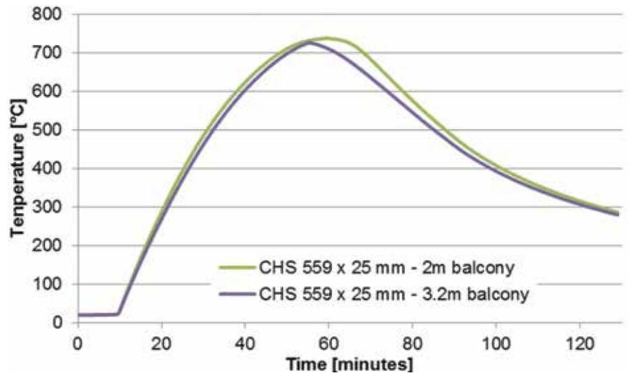
Figure 6. Temperature – time profile within external bracing due to compartment fire (Source: BuroHappold Engineering)
