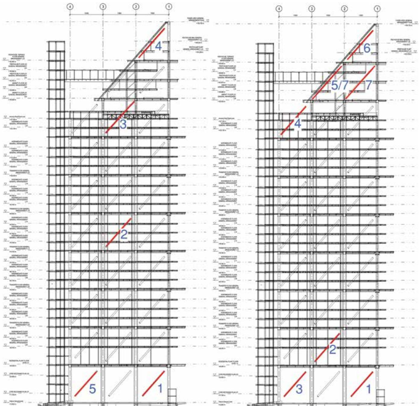
Figure 9-10. Diagonals subject to heating as part of the thermal expansion analyses (left); Diagonals removed as part of the redundancy analyses (right) (Source: BuroHappold Engineering)
