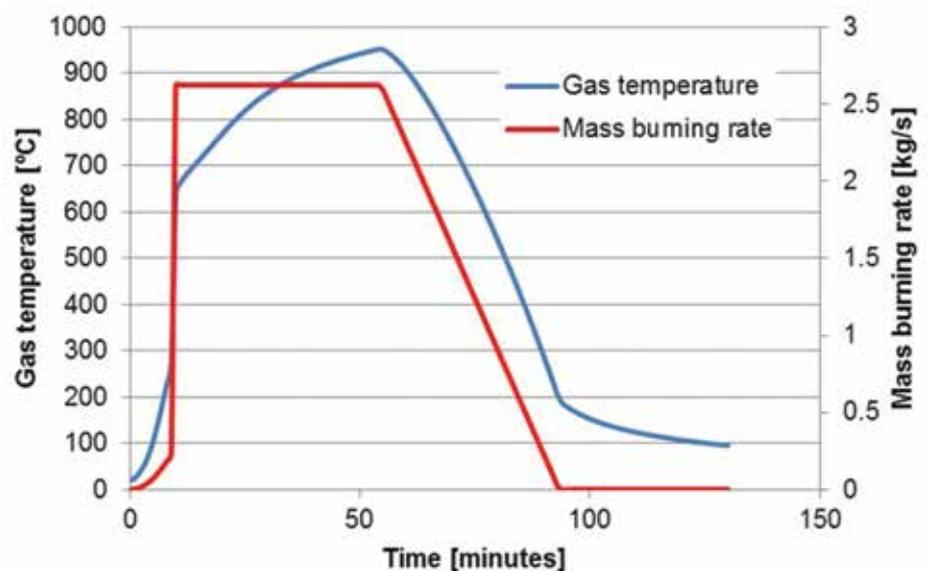
Figure 4. Main results of the worst case realistic compartment fire (Source: BuroHappold Engineering)
