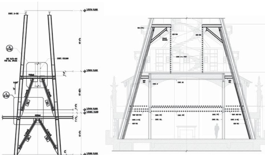
Figure 8. Pinnacle reinforcement.
