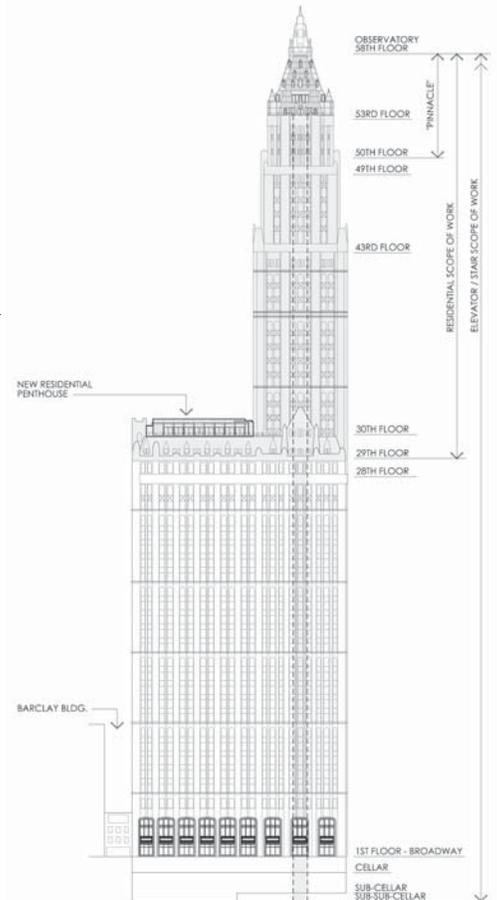
Figure 2. Scope of reconstruction work. © SLCE Architects
