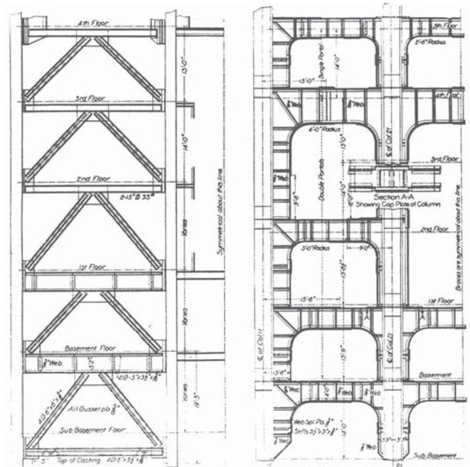
Figure 5. Detail of as-built bracing systems (1913). © Gunvald Aus
