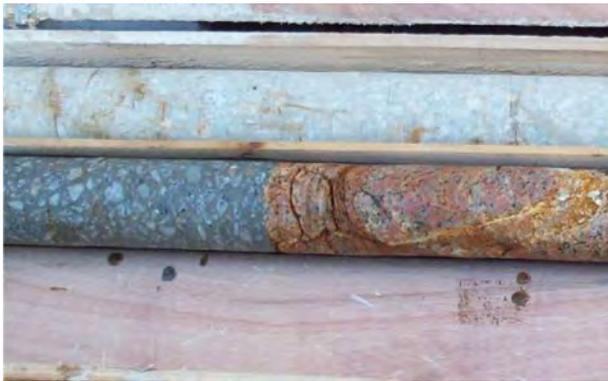
**Figure 4.** Concrete/bedrock interface.
