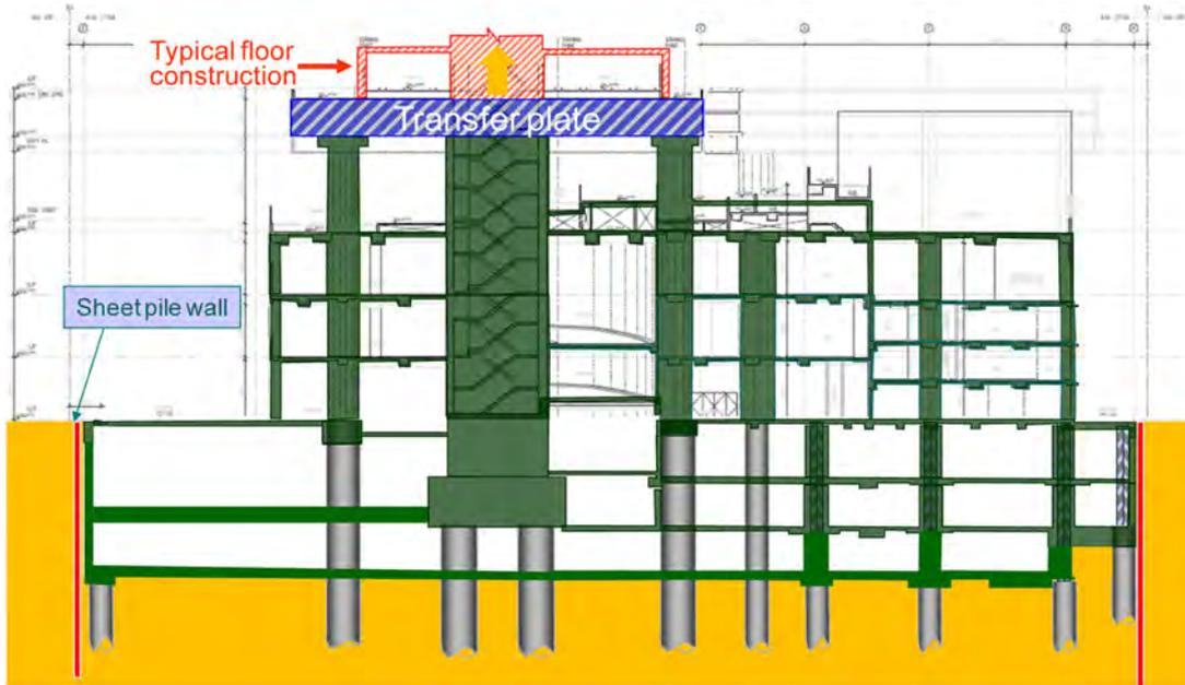
Figure 17. Typical Cross-section along N-S direction.
