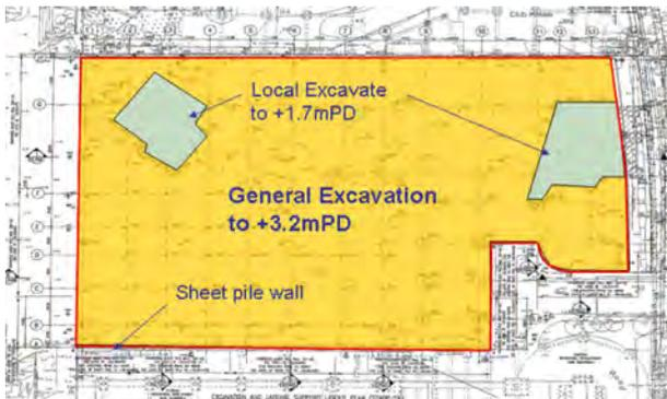
Figure 18. General Excavation near Ground Level.
