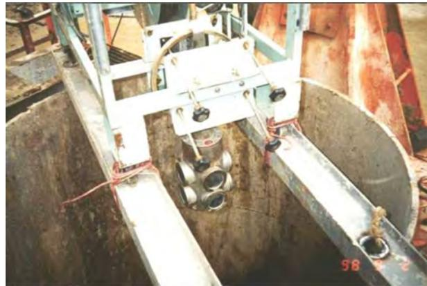
**Figure 2.** Kodon (Sonar) Testing.
