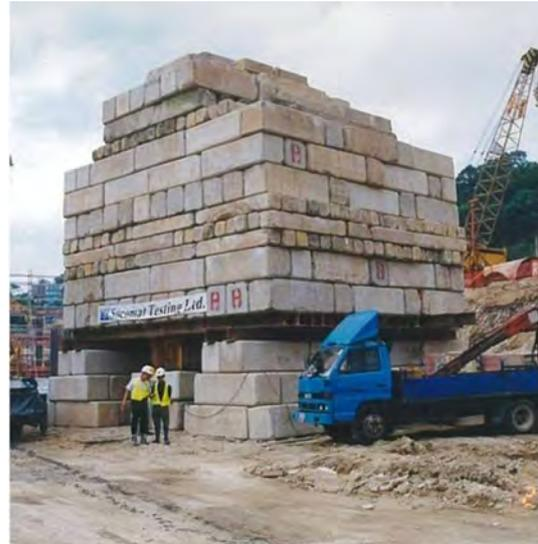
Figure 8. Load test set-up for driven piles.
