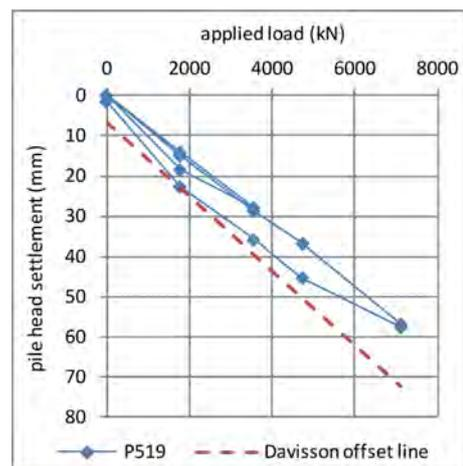
Figure 9. Load versus settlement curve.
