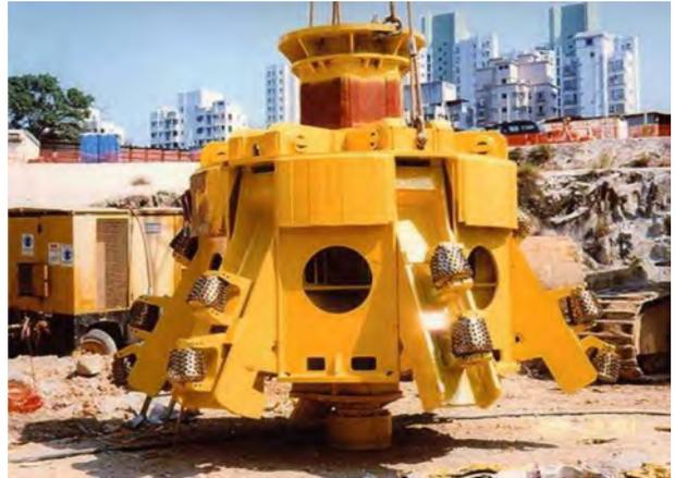
Figure 16. bell-out drill bit.
