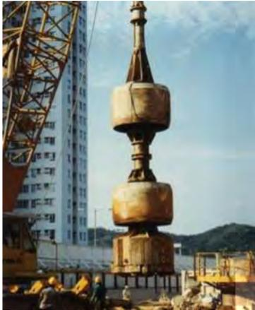
Figure 15. Large diameter RCD drillbit.
