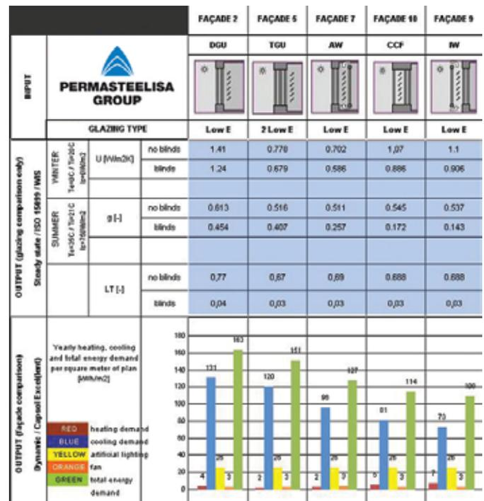
Figure 7. Impact in building energy consumption by using different types of curtain wall at south orientation for Shanghai climate. © Permasteelisa Group
