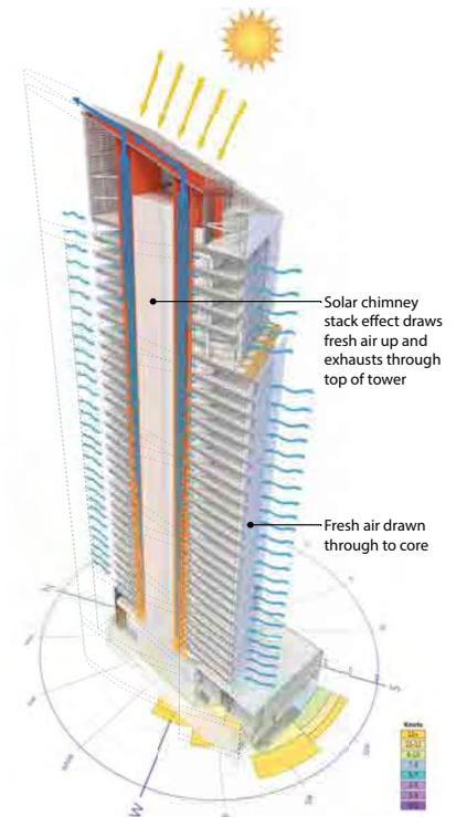
Figure 6. Passive natural ventilation strategy, showing thermally activated solar chimney and shafts connected with user-controlled double façade. © Gensler
