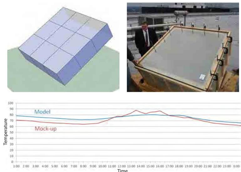
Figure 3. Solar chimney mockup. © Gensler and Buro Happold
