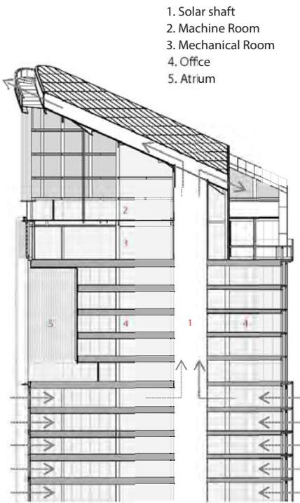
Figure 5. Detailed section of the solar chimney. © Gensler
