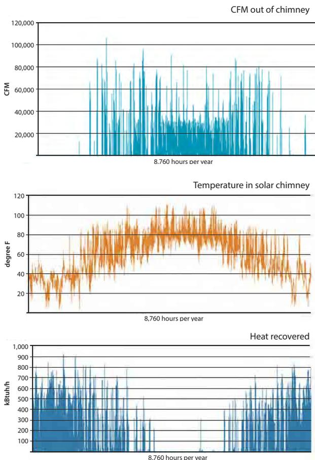
Figure 2. Solar chimney simulation. © Gensler and Buro Happold
