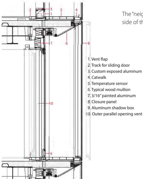
Figure 9. Double façade detail. © Gensler
