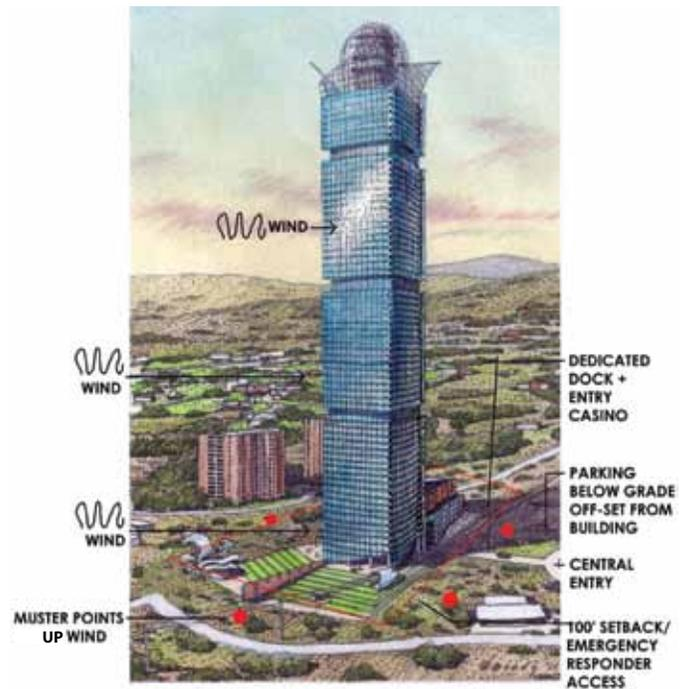
Figure 6. Allocating the muster points © Yas Architecture
