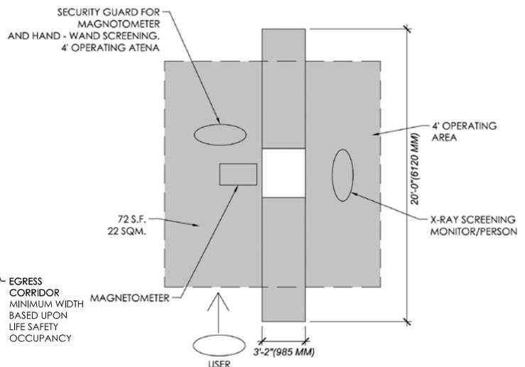
Figure 3. Space allocations for a typical security point
