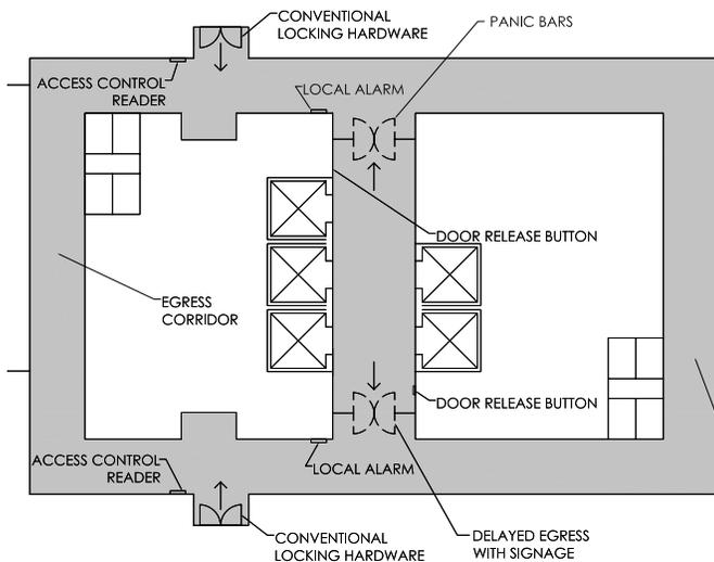
Figure 2. Typical diagram of a secured egress
