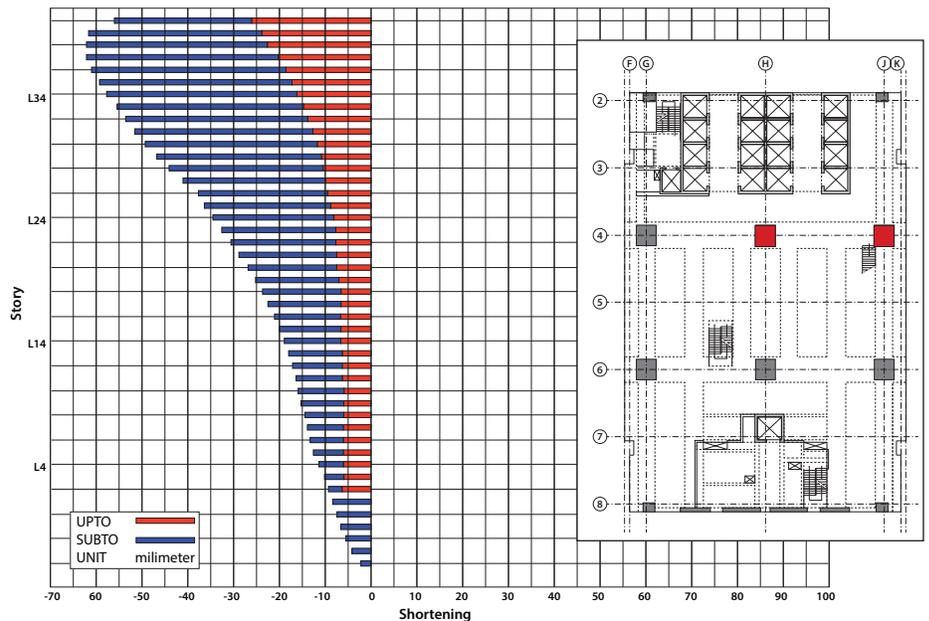
Figure 10. Differential shortening between column H4 and wall J4 of Public Mutual Tower at 100 years.
