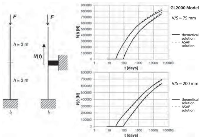
Figure 2. ASAP software validation – case study of a column loaded at time  $t_0 = 7$  days subjected to the application of an additional delayed restraint at mid-height, at time  $t_1 = 28$  or  $t_1 = 90$  days. The graph show the development of the vertical reaction of the delayed restraint for different sets of influencing parameters.
