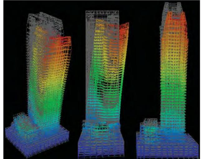
Figure 7. Deformed shape of the Public Mutual Tower at target time of 100 years.
