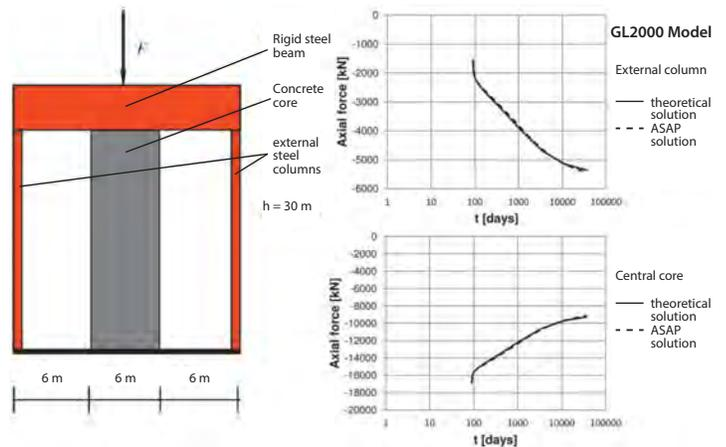
Figure 3. ASAP software validation – case study relative to a non-homogeneous hybrid structure with concrete core and steel columns loaded at time  $t_0 = 90$  days (the horizontal bracing element is considered as a rigid body). The graph show evolution over time of the axial force in columns and core.
