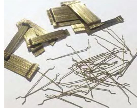
Figure 12. Dramix® steel fibers.
