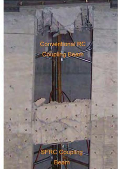
over larger areas of the beam. This can be partly attributed to the ability of the steel fibers to increase the tensile strength of the concrete, raising the force threshold at which spalling occurs (see Figure 10).
