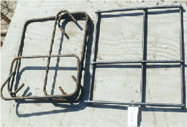
Figure 2 – Photo showing conventional reinforcement on left, WRG on right. (Baumann Research and Development, 2000)
