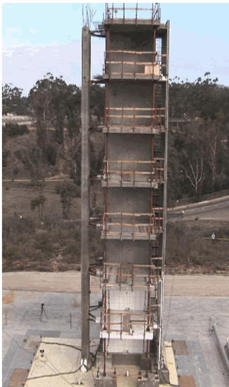
Figure 5. 7-story apartment module on shake table at UCSD's Englekirk Engineering Center (Baumann Research and Development, 2006)
