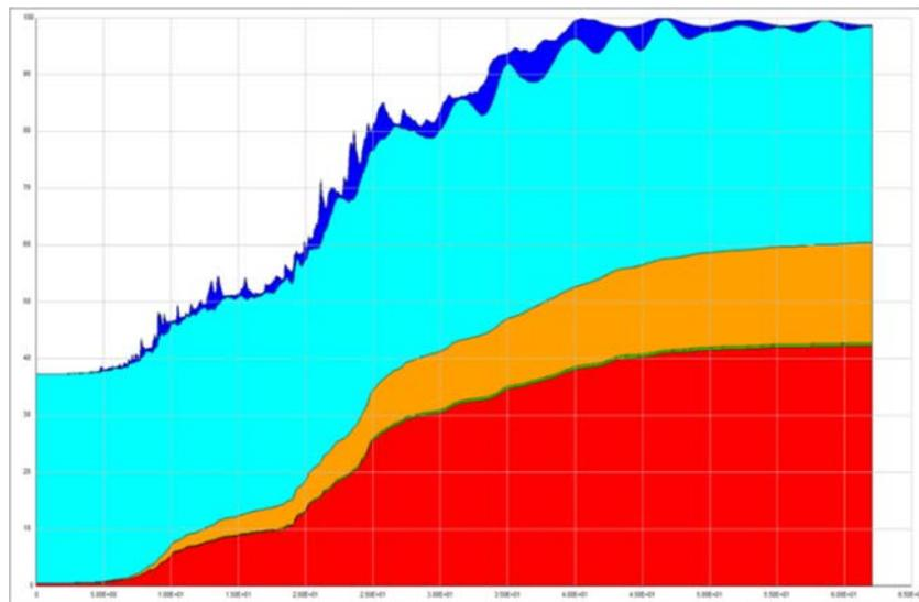
Figure 13. Energy balance for structure.
