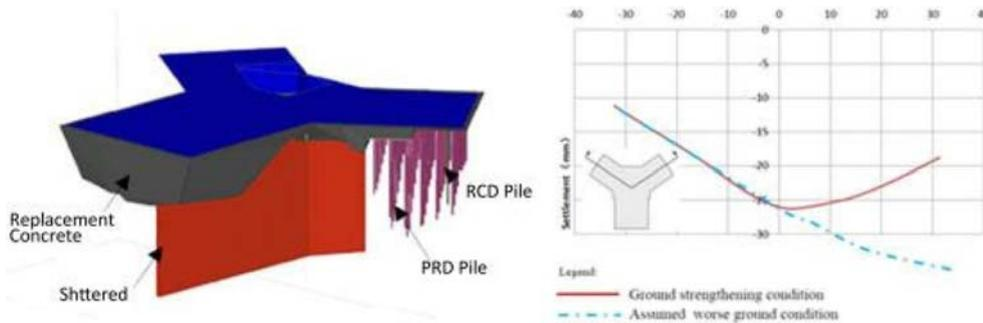
**Figure 7.** Analysis modeling of foundation and displacement of foundation.
