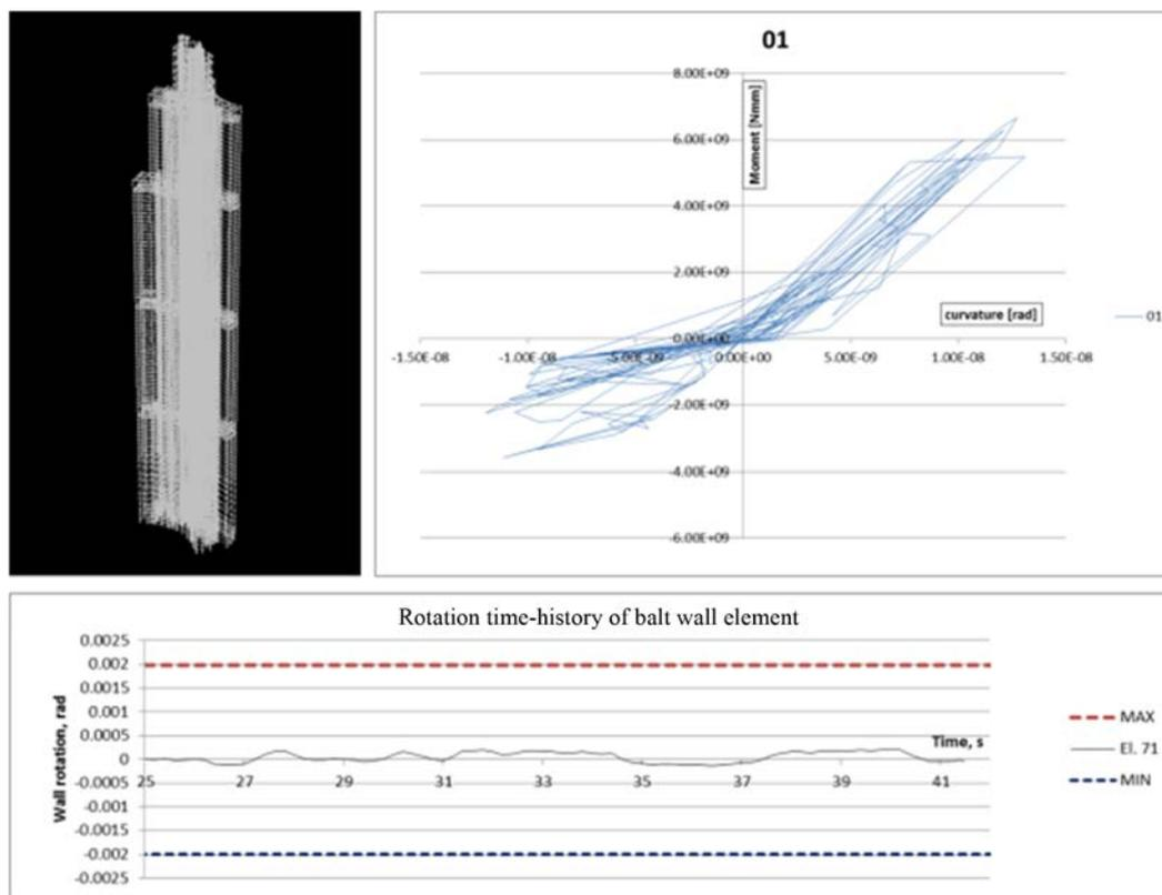
Figure 11. Nonlinear analysis model an result of belt-wall.
