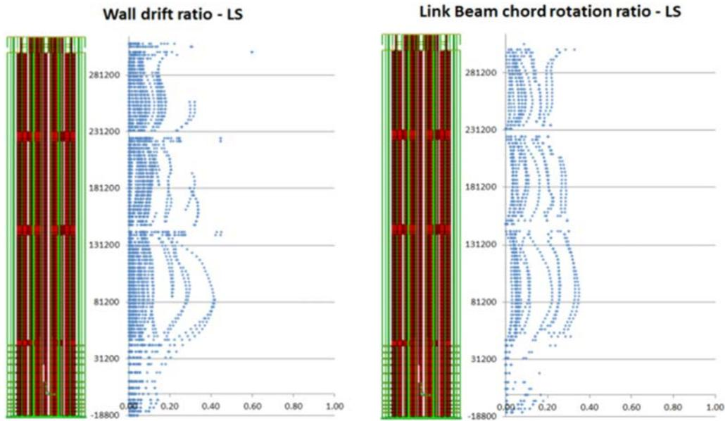
Figure 12. Nonlinear analysis model an result of wall drift & link beam.
