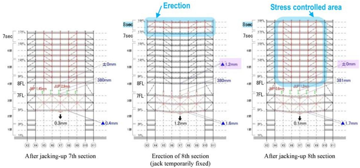
Figure 8. Method of erection above the Mega-truss and displacement control.
