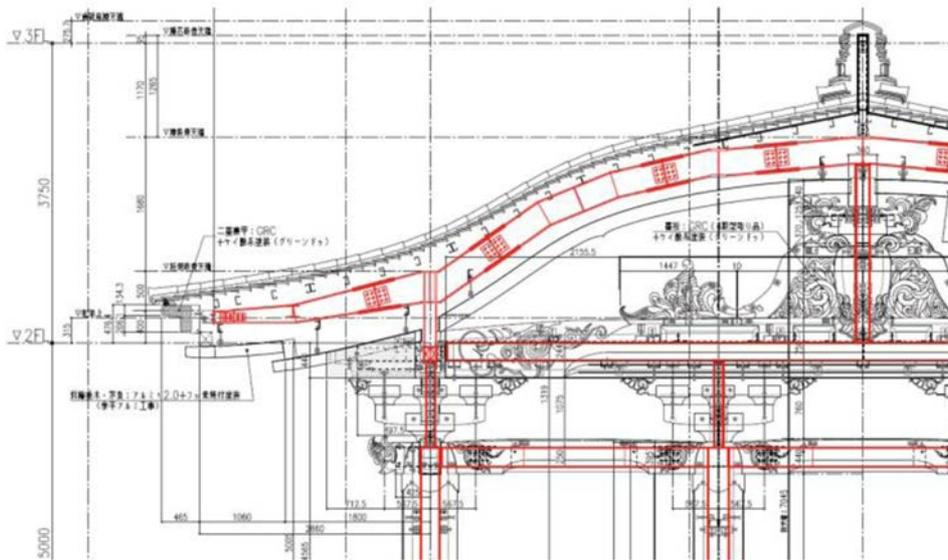
Figure 10. Details of Karahafu-style gable and concealing the structural steelwork.
