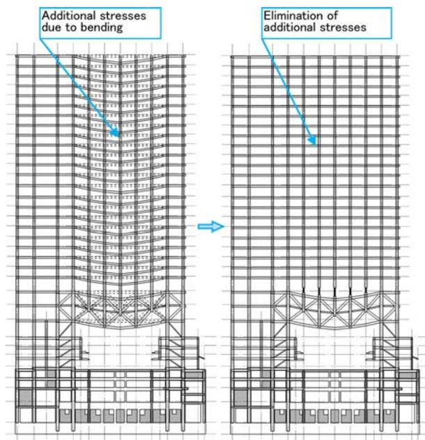
**Figure 7.** Elimination of additional stresses by jacking.
