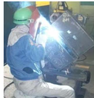
**Photo 5.** Welding test (inclined vertical).
