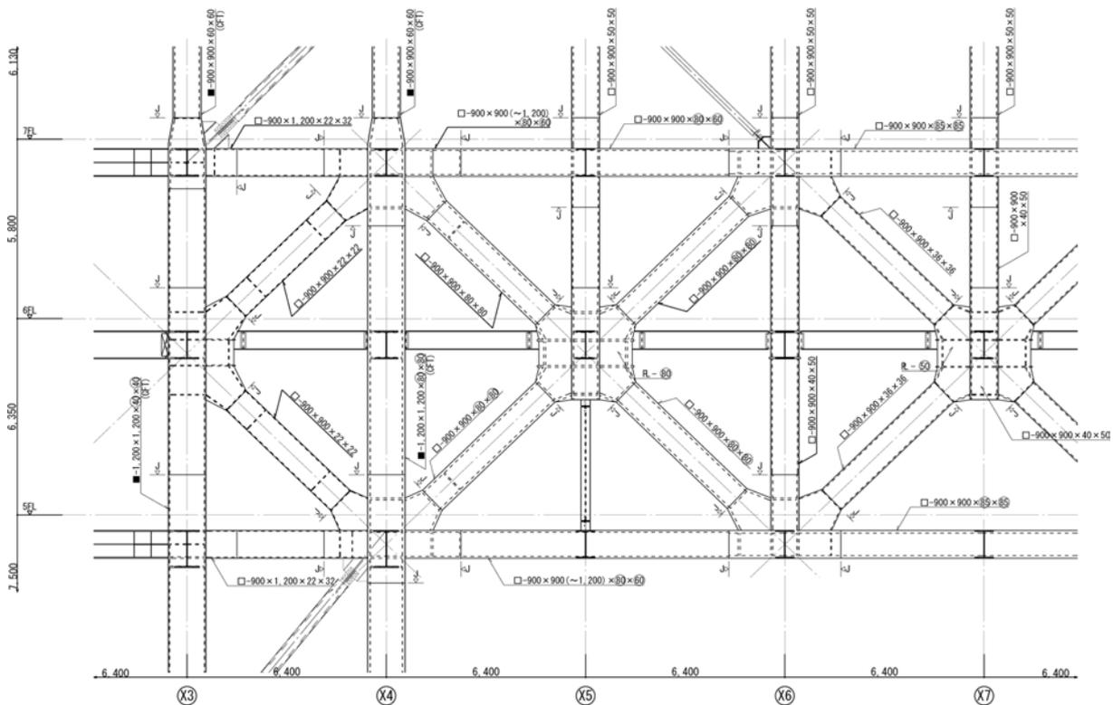
Figure 6. Detail of Mega-truss (Y7).
