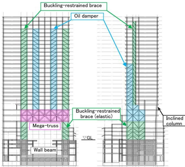
Figure 3. Y7 Elevation.
