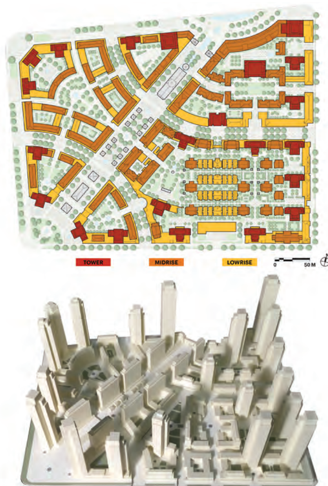
Figure 11. A complex system of streets, blocks, and squares combines with a hierarchy of building heights to create an ordered but varied community. (Source: RAMSA)
