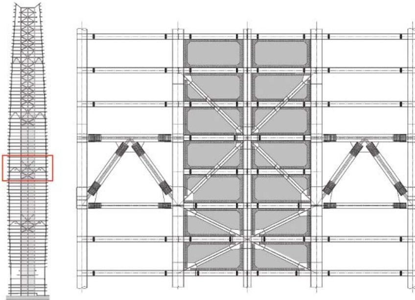
Figure 4. Outrigger truss
