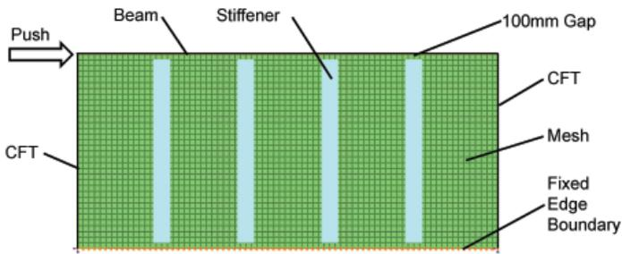
Figure 9. SPSW pushover model and deformed shape
