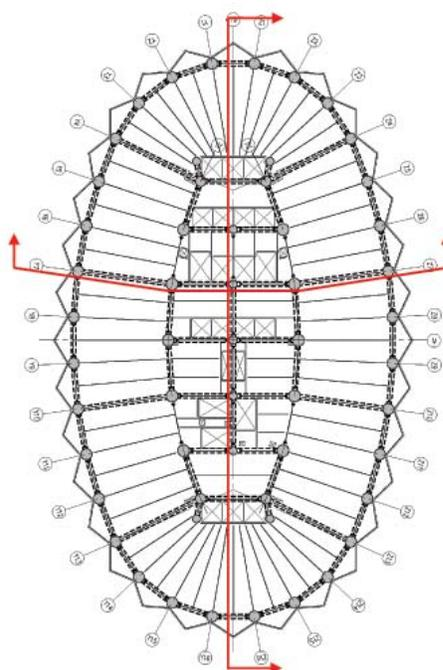
Figure 3. Structural plan at outrigger levels and overall building sections
