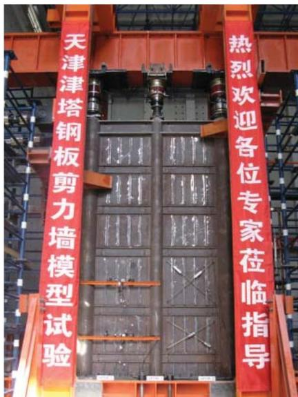
Figure 10. SPSW assembly test set-up
