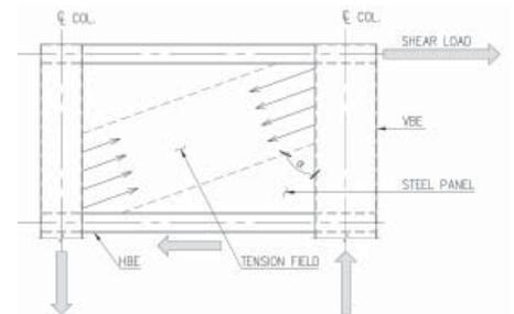
Figure 6. Tension-field action
