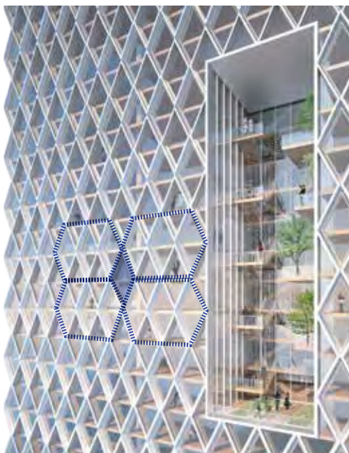
Figure 12. Duplex module connection configuration. © Perkins+Will
