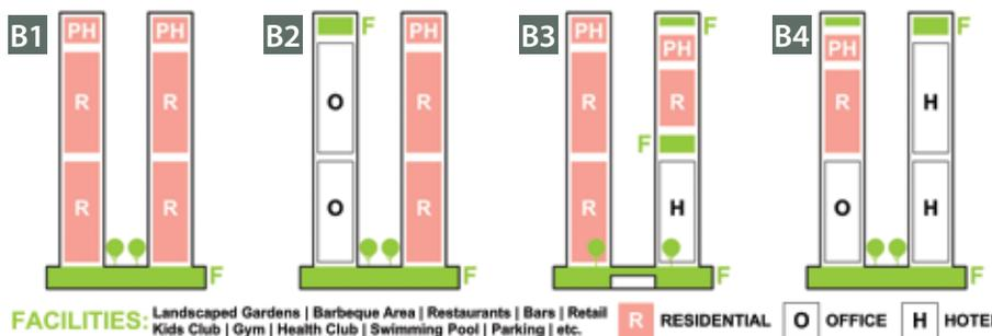
Figure 5. Examples of two-tower complexes in Group B: (from the left) 29 Boulevard Complex, Churchill Towers, Grosvenor House Complex, and the Sofitel Dubai Downtown & Burj Gate 48 Complex.
