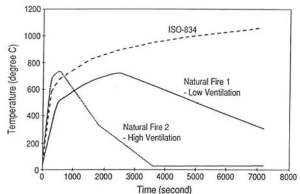
**Figure 6.** Comparison of temperature-time curves of ISO standard fire and natural fires. (Richard Liew et al., 1998).
