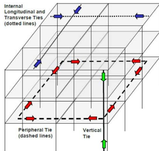
**Figure 2.** Tie forces in a framed structure (DoD, 2010).
