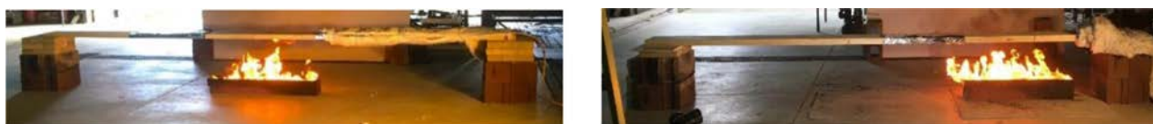
Figure 5. Test setup of the heating portion of the experiment for the moment region (left) and the shear region (right).
