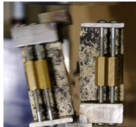
Figure 8. Typical failure mode of shear along an adhesive bond line.
