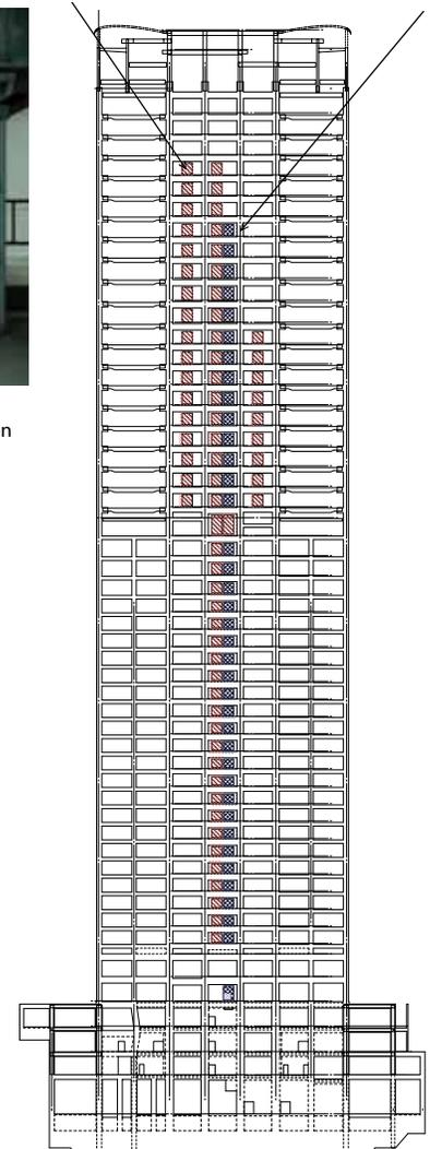
Figure 17. Section showing location of damping equipment at Ark Hills Sengokuyama Mori Tower, Tokyo. © Obayashi Corporation
