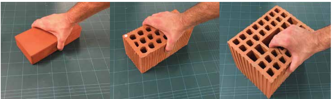
Figure 5. Bricks (like many building materials) have evolved adapting themselves to the human worker that assembles them. It is nonsense to build a robot to assemble brick walls: if they don't have to be assembled by humans, bricks can have other shapes, sizes, and weights.
