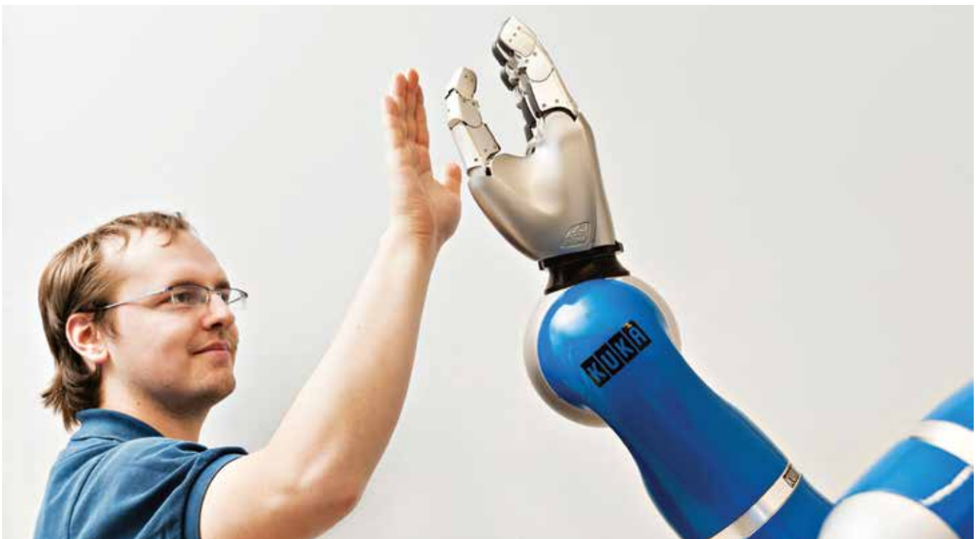
Figure 4. Co-Bots (collaborative-robots) are robots that can work in a mixed environment with humans, thanks to their smaller size, slower speed, and special sensors to avoid injuries. © Daimler und benz Stiftung (cc by-sa)
