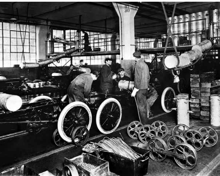
Figure 1. The Ford model T assembly line is the prototype of industrial production. Hordes of workers do the same task all day long, while the car being assembled advances through the factory.
