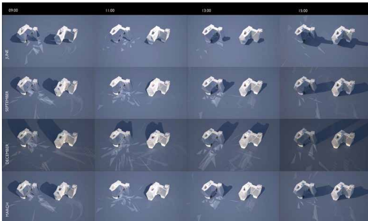
Figure 10. Reflectivity and shading analysis. © Ron Arad Architects
