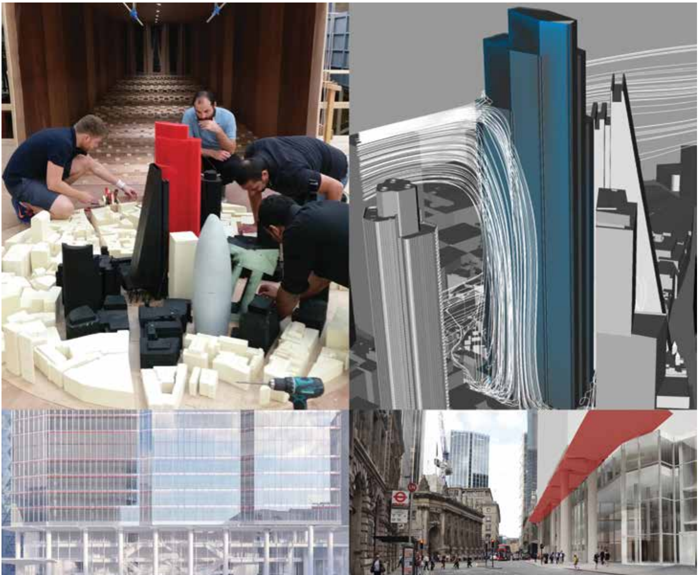
Figure 6. 22 Bishopsgate, Wind testing and analysis for mitigation and pedestrian comfort. Wind tunnel test at RWDI (top left). Downdraft analysis by Wirth Research (top right). Bishopsgate main foyer elevation (bottom left). Perspective diagram of the UHPFRC canopy in the context of the Bank Conservation Area (bottom right). © RWDI (top left, top right); Martin Richardson (bottom left); PLP Architecture (bottom right)
