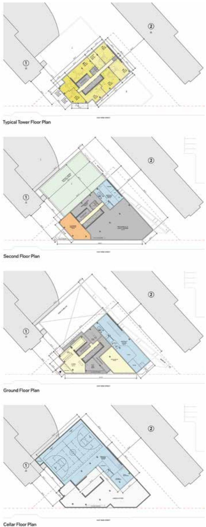
Figure 7. Typical floor plans of The Bellwether, from bottom to top: cellar, ground floor, second floor, and typical tower floor. © FXCollaborative
