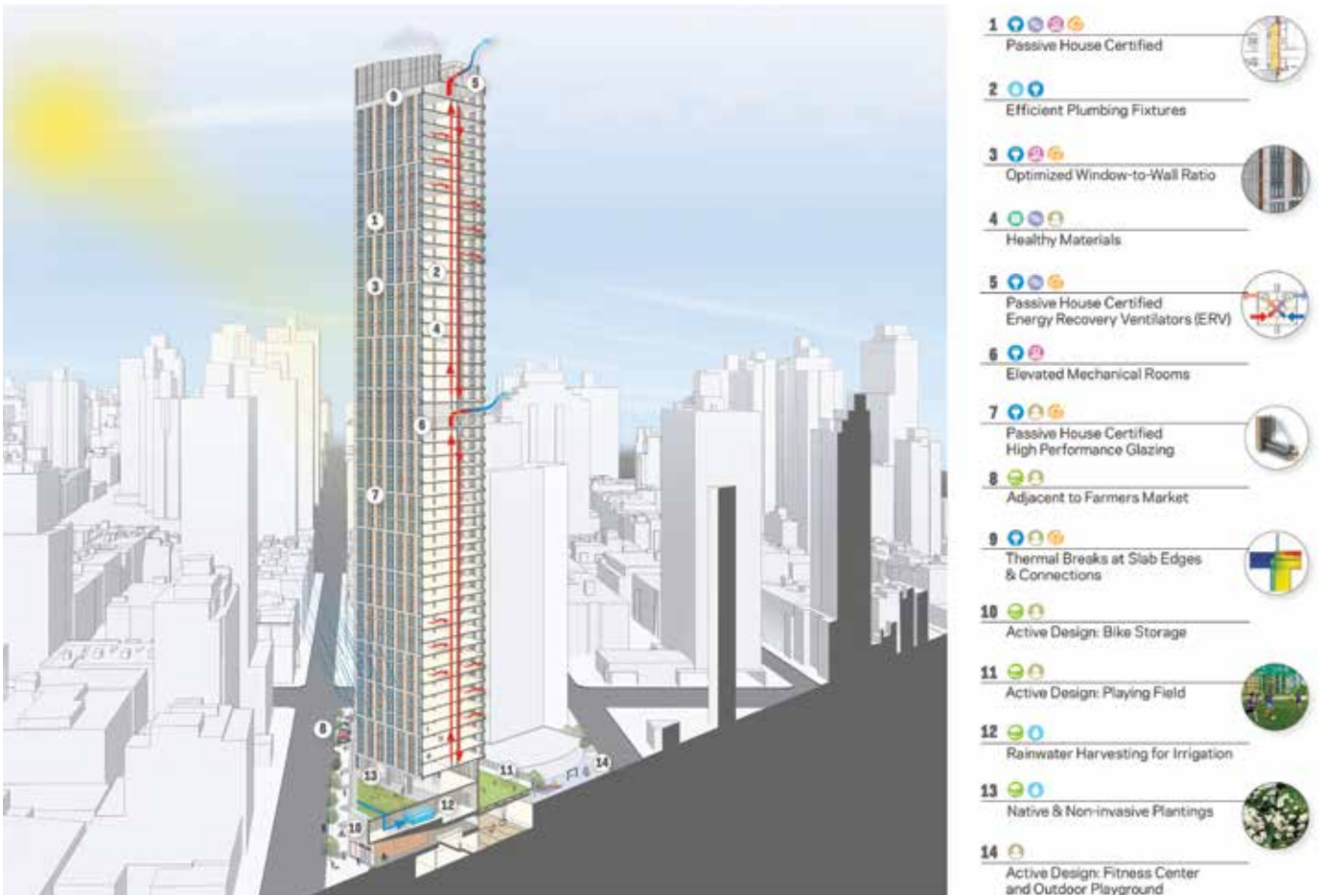
Figure 10. Sustainability diagram of The Bellwether showing the incorporation of sustainable elements into the architectural design. © FXCollaborative
