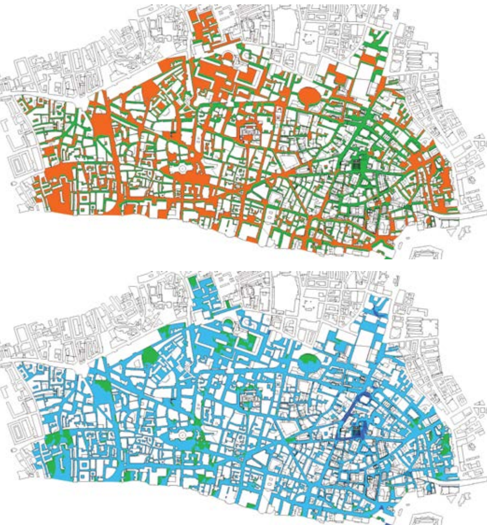
Figure 5. UTCI comfort conditions in the Square Mile during summer (top) and winter at midday (bottom). © RWDI
