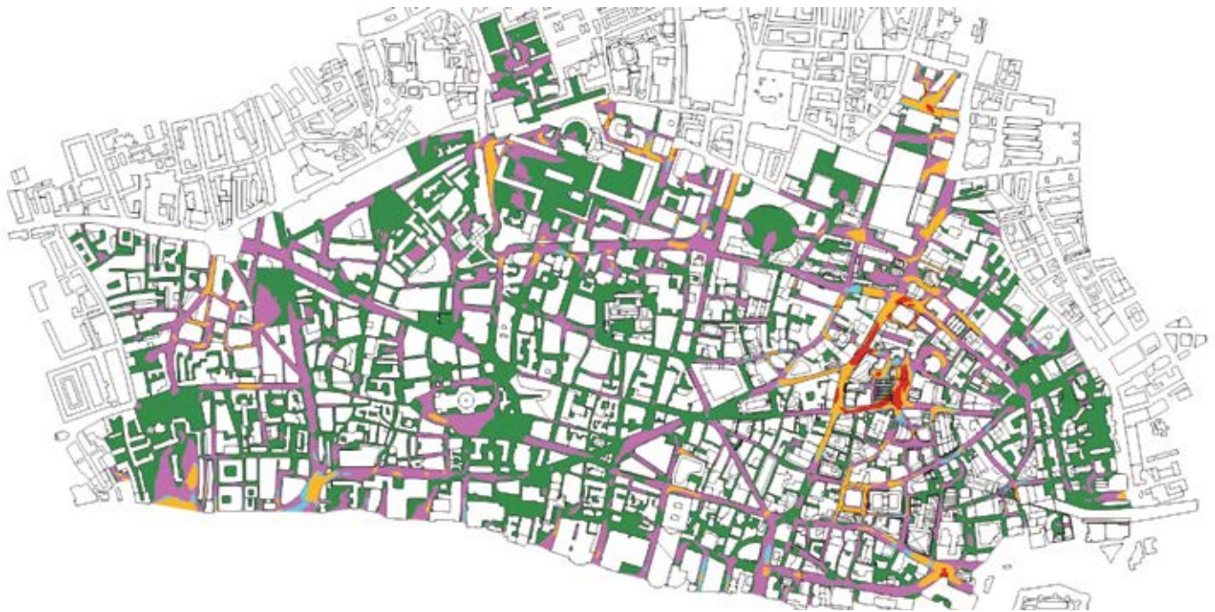
Figure 6. Contour plot showing the thermal comfort conditions, using the modified UTCI categorization developed for the City of London. © RWDI
