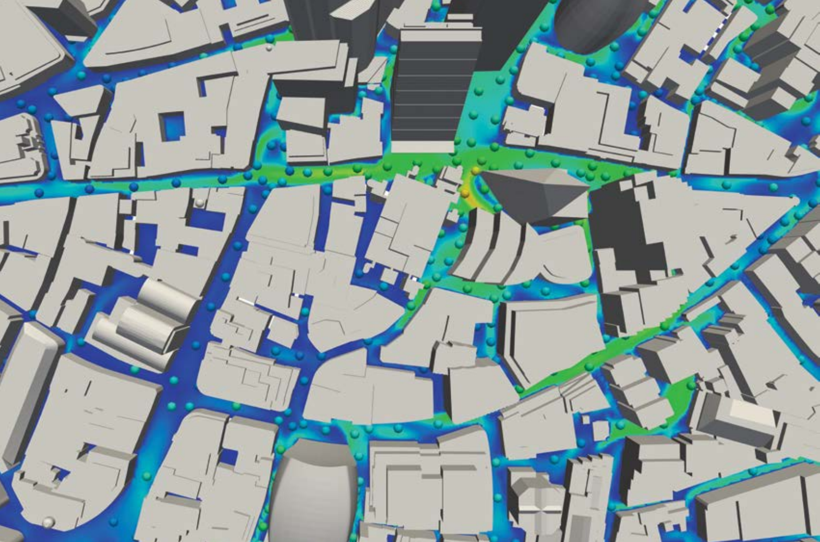
Figure 2. A comparison of wind comfort conditions around the Eastern Cluster, as obtained from CFD simulations (continuous color contours) and wind tunnel tests (discrete color-coded dots). © RWDI
