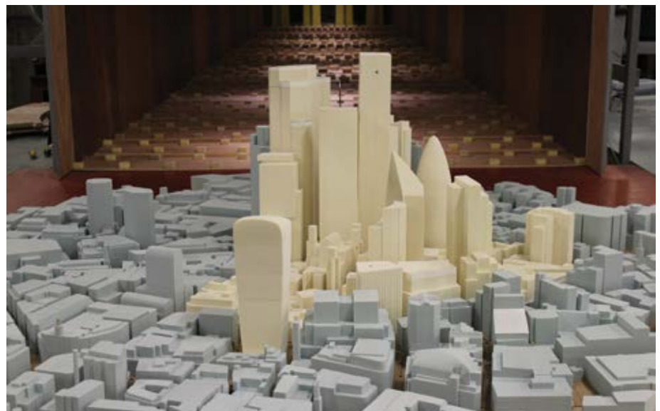
Figure 4. Flow visualization showing the so-called “huddled penguin effect” that is created by the collective impact of all tall buildings (top). The City of London model at RWDI's wind tunnel (bottom). Both types of models are now used to substantiate the City's microclimate guidelines. © RWDI
