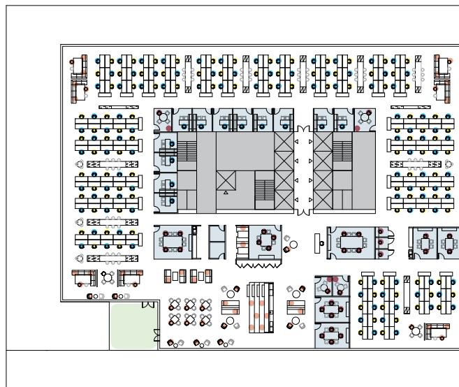
Figure 7b 245 SF (22.7 m 2 )/PP 26,520 USF (2,460 m 2 ) 265P Max Occupancy 89:11 Ratio WS/Office 1:0:8 Task Seat to Collab Seat
