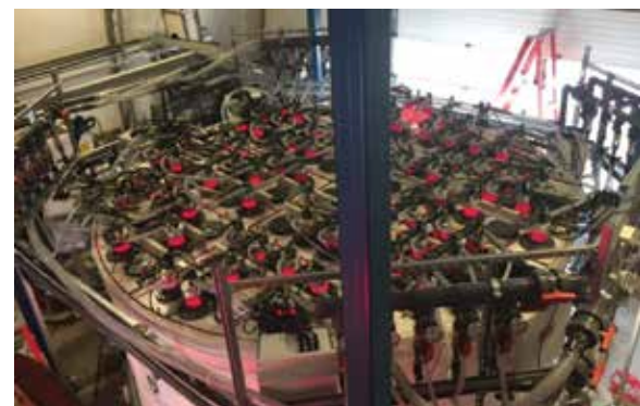
Figure 12. An algae bioreactor tank. Carbon dioxide (CO 2 ), nitrogen oxides (NO x ) and sulphur oxides (SO x ) are injected into a carbonized column inside the water tank, acting as a feedstock for the blue-green algae when combined with a highly-efficient LED lighting system to stimulate photosynthesis. © Pond Technologies Inc.
