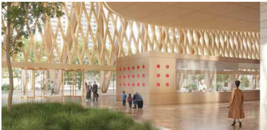
Figure 13. Algae bioreactor in ground-floor lobby. Part of the bioreactor is exposed in the lobby, allowing light to shine through light portholes, revealing the algae growing in response to light and emissions from the natural gas cogen plant, as part of a "science on display" education strategy.
