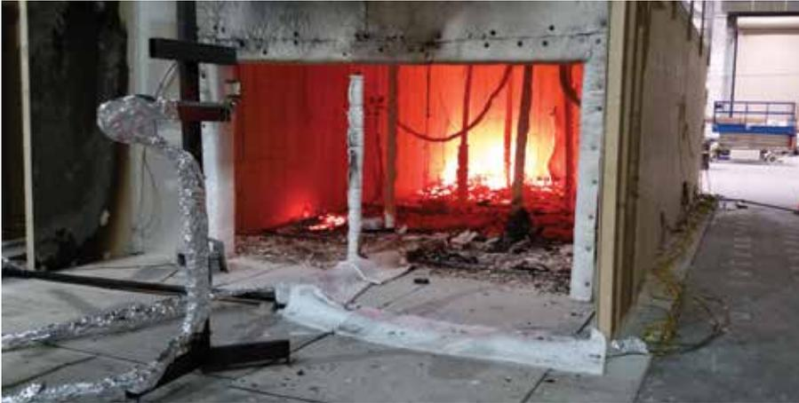
Figure 8. CLT compartment fire from the Fire Protection Research Foundation series of tests.
