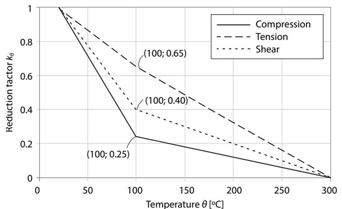
Figure 5. Reduction in compressive strength parallel to the grain in softwoods, plotted against rise in temperature. Source: BS EN 1995-1-2, 2009
