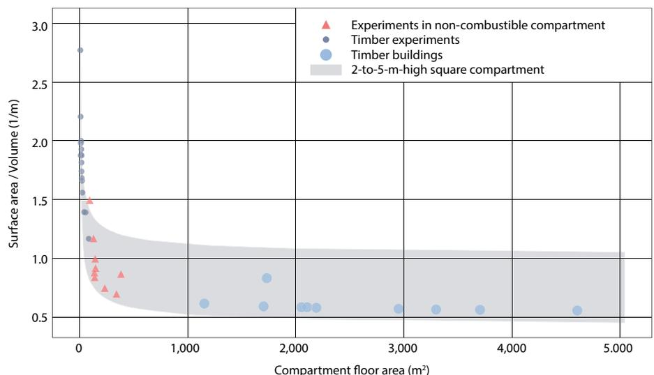
Figure 10. Graph illustrating the discrepancy between the available timber compartment fire tests and the proposed or constructed high-rise mass timber buildings.
