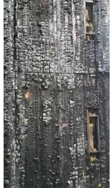
Figure 7. CLT panel, showing char fall-off after a standard fire test.
