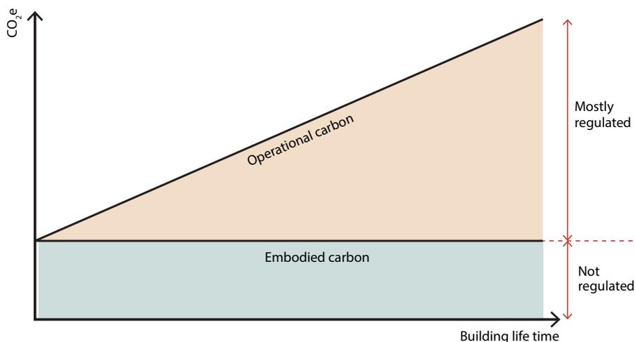
Figure 1. The level of embodied carbon in buildings is largely unregulated. Use of timber in building structures can help limit embodied carbon emissions.
