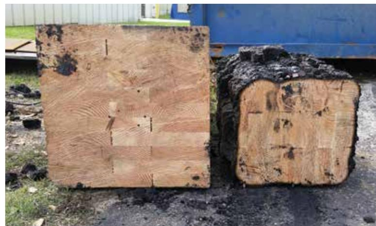
Figure 3. Glulam column, before and after a 90-minute fire-resistance test, showing extent of reduced cross-section.
