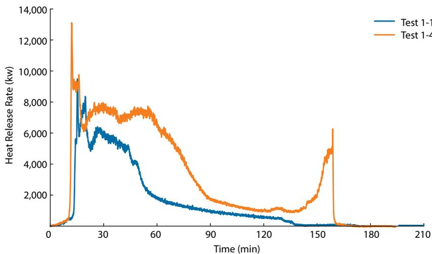
Figure 6. Compartment fire with comparison of heat release rate. Test 1-1 has no timber exposed, and Test 1-4 has CLT exposed at the ceiling. Tests were stopped with manual intervention. Source: Su et al. 2018
