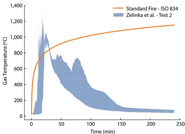
Figure 4. Graph showing the difference between the standard fire (CAN/ ULC S101) and the temperatures from a compartment fire (natural fire curve). Source: Taber et al. 2014
