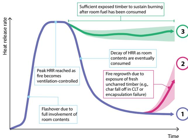
Figure 2. General trend lines of heat release rate (HRR) vs. time plots from experimental data of ventilation-controlled fires within exposed CLT compartments.
