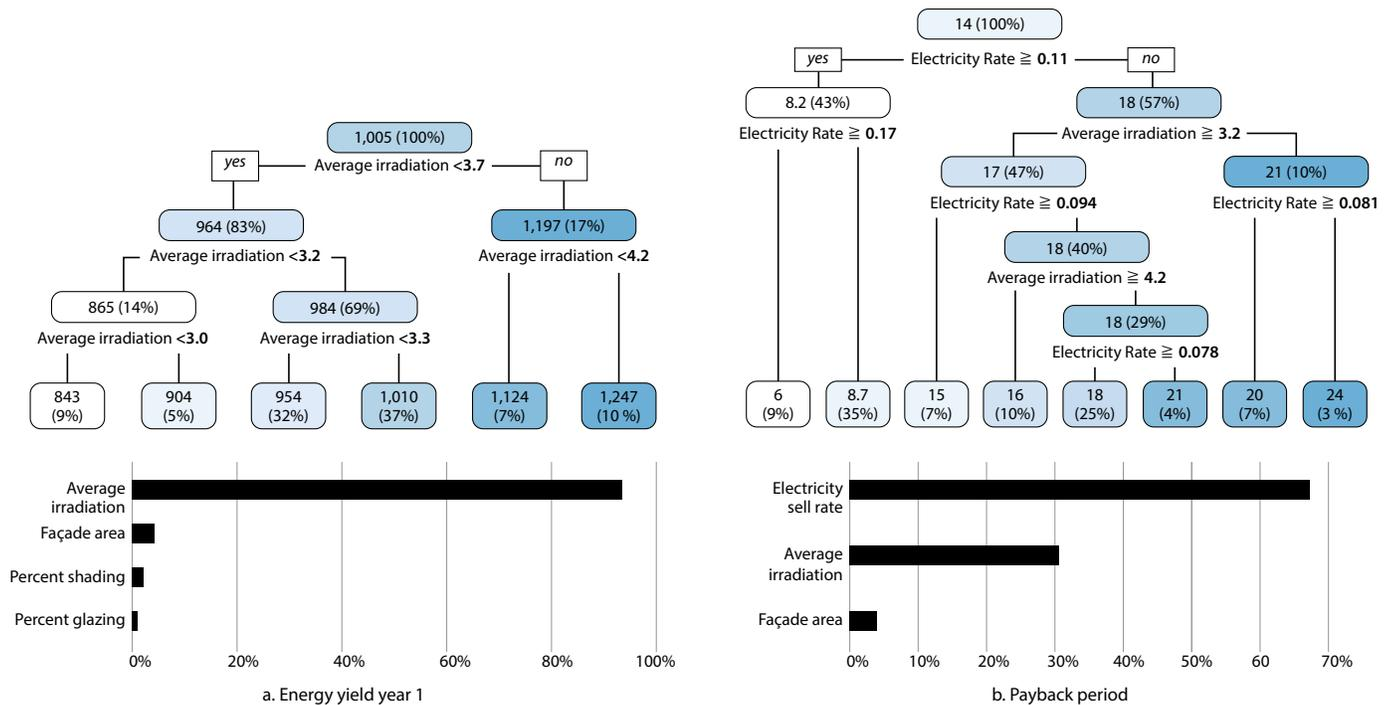
Figure 6. Result of classification and regression tree analysis. Model (a), at left, examines the effect of monthly average solar irradiation, façade area, and glazing percentage on energy yield. Model (b), at right, compares the amount of influence irradiation levels, electricity rates, and façade area have on time to payback of an investment in BIPV panels.
