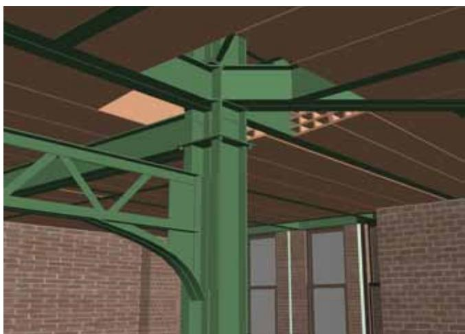
Figures 5 & 6. Digital reconstructions showing the hybrid of masonry piers and cross-walls with steel columns, girders, and portal frames. © Shaghayegh Missaghi and Ryan Gauquie
