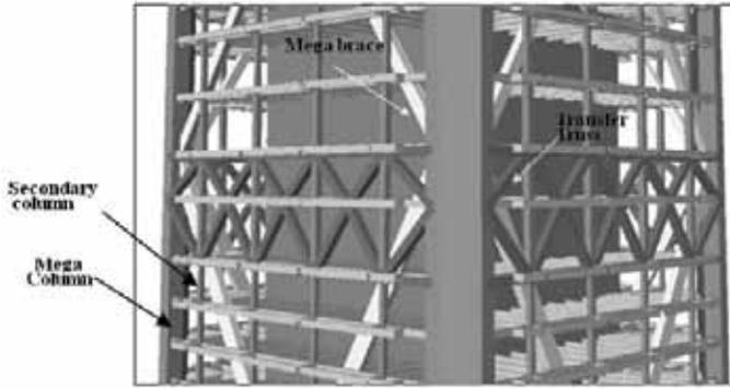
Figure 5. Illustration of Mega Frame and Mega Brace connection – double-story truss
