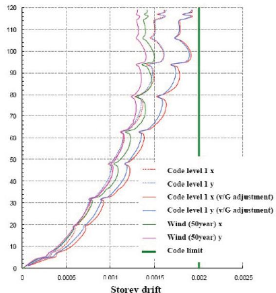
Figure 10. Inter-story drift under earthquake and wind
