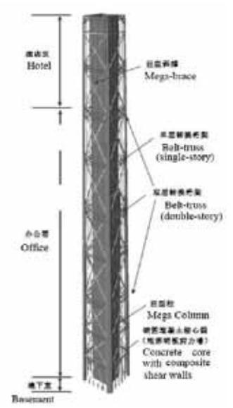
Figure 3. 3D Illustration of Structural System
