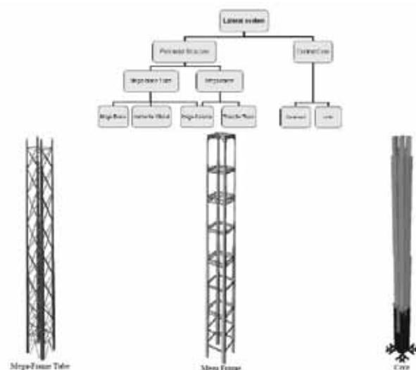
Figure 4. Dual Lateral Stability System
