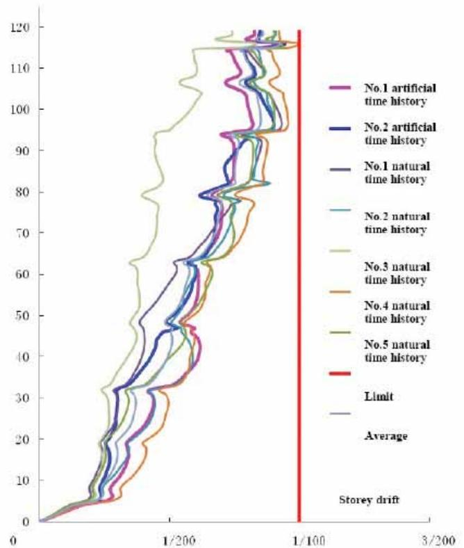
Figure 12. Overall inter-story drift under severe earthquake elastic-plastic time-history analysis
