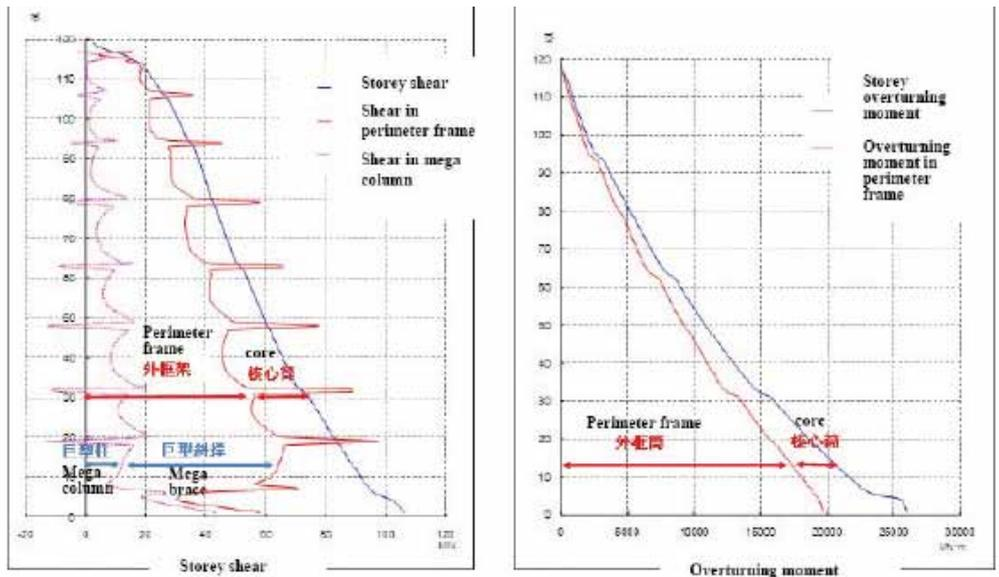
Figure 11. Distribution of shear and overturning moment between internal and external frame
