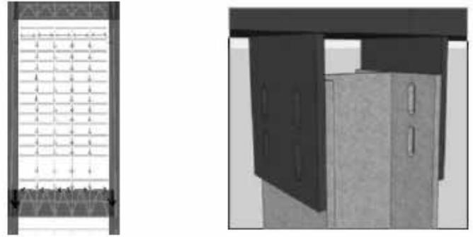
Figure 6. Elevation of perimeter frame and slotted joint at the top
