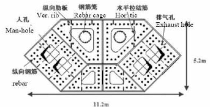
Figure 8. Typical low zone 45m² Mega Column section detail
