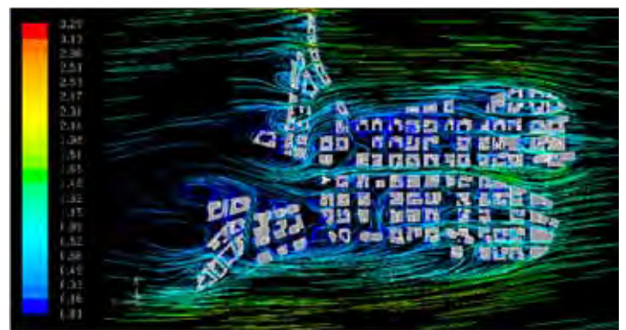
Figure 12. vector of velocity in the 1.5m height (m/s) 图12. 1.5米高速度分布 (m/s)
