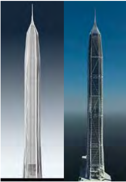
Figure 4. The form and structure of PAFC share a high degree of affinity. (Source: KPF and Thornton Tomasetti) 图4. 平安金融中心造型与结构高度关联 (来源: KPF与Thornton Tomasetti)
